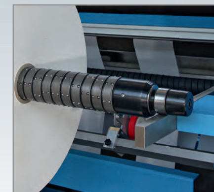
Dynamic support of winding shafts
